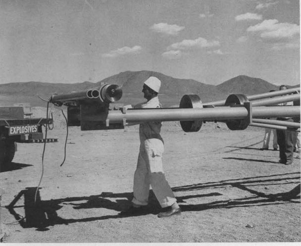
EXPLOSIVE CHARGES on the rocket centrifuge are adjusted by Paul Syroid, division supervisor of the Specific Projects Division, 1613, in preparation for acceleration test. Rocket centrifuge is acceleration test machine for components and systems, whirls them about to test their performance during increasing acceleration forces. Sandia scientists attain accelerations on this machine numbered in thousands of G's. \_\_\_\_
